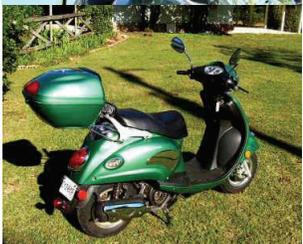
With both mounting clamps attached, you have a strong trunk unit attached to your scooter. There will be plenty of room to remove the gas cap and fuel your scooter. If there are any cautions about this installation, it is to be very sure the front clamp rail lip passes over the front cross-member of the chrome rack. That,
