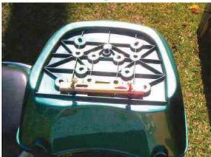
2A - Open the trunk box and insert two long 8mm screws with a washer in the front hole set. Use masking tape to hold them in place by taping over those screws and washers inside. Close the trunk, and turn it upside down as shown. Next, place a clamp bar over the screws with the open ridges of the bar facing down. Place a flat washer on, then a lock washer. Start a nut on each bolt. Only screw the nuts on a couple turns. You only want them loosely attached at this stage.
