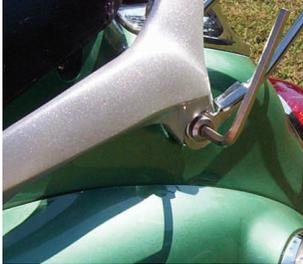
1. The first step is to remove the existing seatback assembly bar, on the QT-2 scooter that is attached with 4 ea. 6 mm screw bolts to the scooter. You do this with the hex wrench supplied in your scooter toolkit. Other models need no rack.
